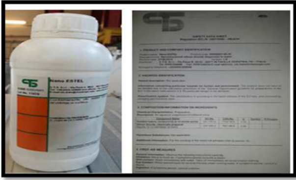
Fig. 1. Nano-silica “Nano ESTEL” used in concrete mix.
